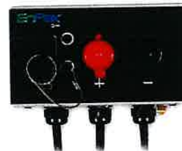
Weld/battery output panel
